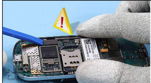
18. Gently lever up the flex connector evenly. Prevent mechanical stress to the components underneath.
